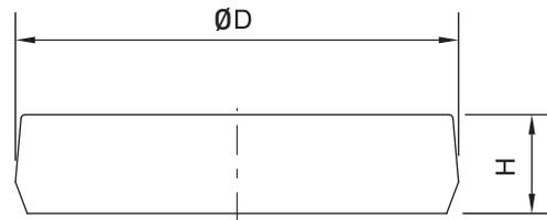
Table 2-8-12 Dimensions of Bolt Caps for Rail Mounting Holes
