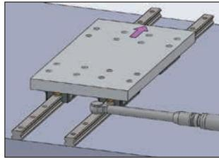
Fig 1.11.16 Compare to the master Linear Guide rail
