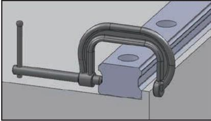
Fig 1.11.13 Mounting the master Linear Guide rail
