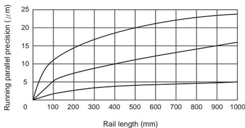
Fig 2.3.6 Running parallel precision slide relative to the rails datum
