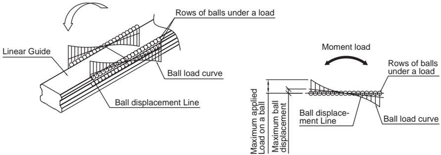
Fig 1.6.1 Ball Load Effectuated by a Moment
