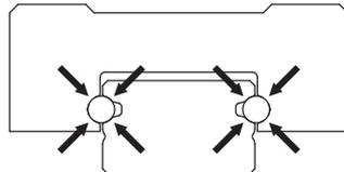
Fig 2.3.4 The Gothic 45° four-direction load structure
