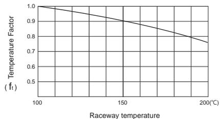
Fig 1.3.3 Temperature Factor (f<sub>t</sub>)
